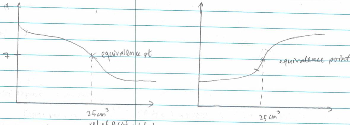
e.g.  $\text{CH}_3\text{COOH}$  (weak acid) and adding  $\text{NH}_3$  (weak base)
